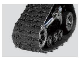
Heavy-duty, wide, rubberized wheels on a UHMW base to distribute the weight of the side-by-side
